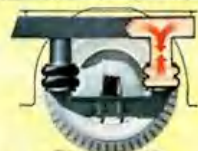
Air Suspension Ride —Entire coach floats on cushions of air, in rubber-nylon bellows.
